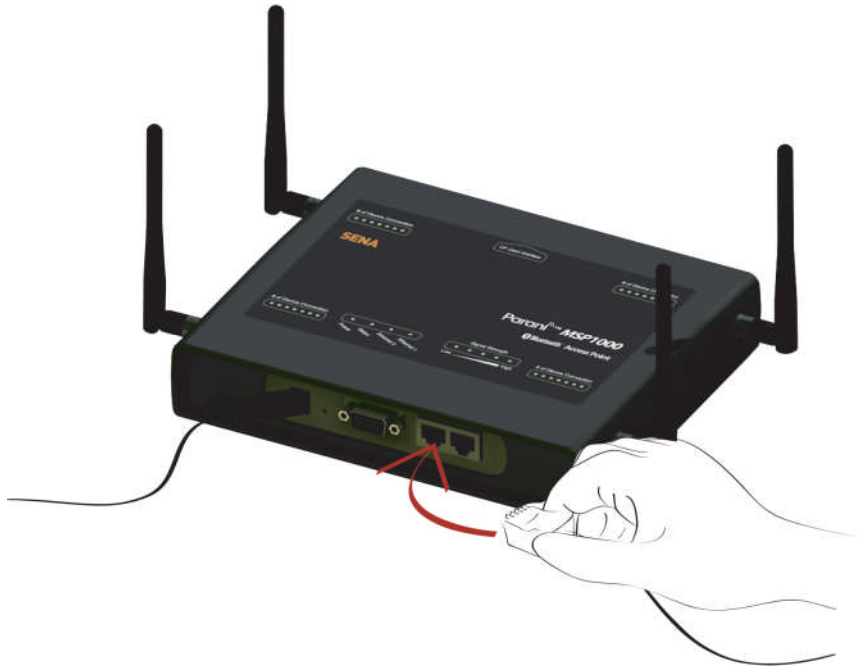
Figure 2-3 Connecting a network cable to the Parani-MSP1000
