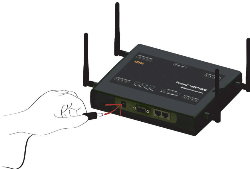
Figure 2-2 Connecting the power to the Parani-MSP1000
