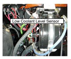
If no coolant or corrosion is found, remove the harness connector from the low coolant level sensor and connect the jumper harness to the coolant level sensor. Loop the excess harness and use tie wraps to secure the loop. Connect the other end of the jumper harness to the engine harness.
