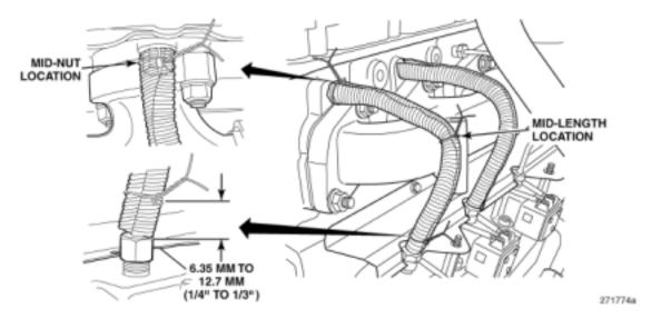
Figure 7 — Securing Sleeve with Safety Wire
