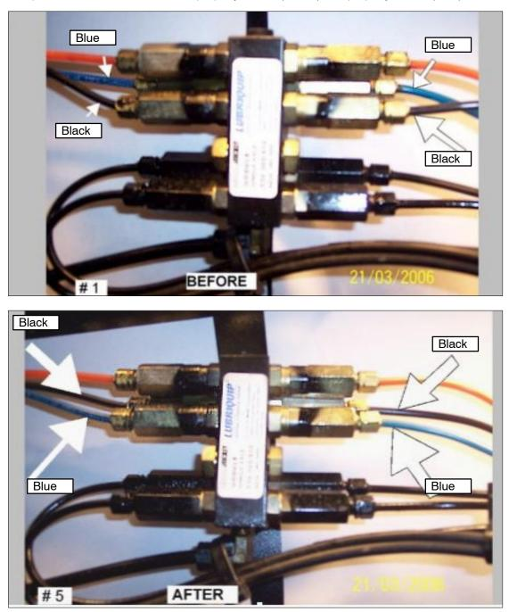
The photos below show the lines improperly routed (before) and properly routed (after).
