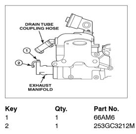
**Description** Screw, M10 x 1.50 x 20 mm long Bracket, breather tube mounting, lower
