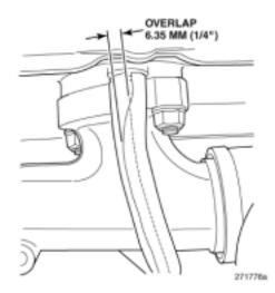
Figure 6 — Overlap Edges of Sleeve
