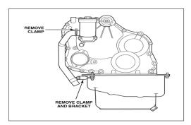
2. Remove the breather canister from the timing gear cover.
