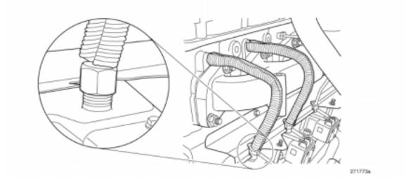
Figure 5 — Aluminum Sleeve Installation (Lower Line Nut End)
