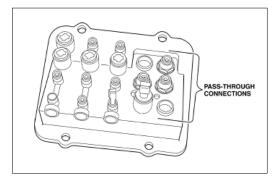
Clearly mark the air lines to identify the air lines connected to each of the pass-through bulkhead fittings and then use the push-to-connect release tool (Weather-head part number 1800TRK) to disconnect the lines from the fittings. The lines must be clearly marked to ensure they are reconnected to the correct ports on the replacement manifold.
