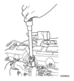
Figure 2 — Proper Use of Injection Line Nut Torque Adapter
