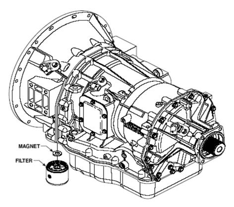
1. Remove the control main filter by rotating it in the counterclockwise direction. Use a standard strap-type filter wrench.
