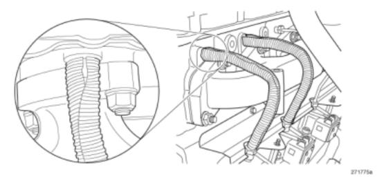
Figure 4 — Aluminum Sleeve Installation (Upper Line Nut End) The lower end of the sleeve must be flush with the line nut, but must not cover the nut hex.
